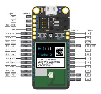
Some pins in the same positions are named differently between the Argon and Photon 2:
