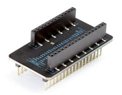
The <u>Particle classic adapter</u> can be used to plug a Photon 2 into a socket that is intended to support an Electron. It can also fit in a Photon socket, however pins will hang past the socket, so there must not be anything in the way, or anything that would short the overhanging pins.
